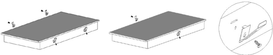
**Fix hob to cabinet:** Insert the hob into the cabinet/work surface as below diagrams, the mounted clips on the sides can secure your hob sturdily.
